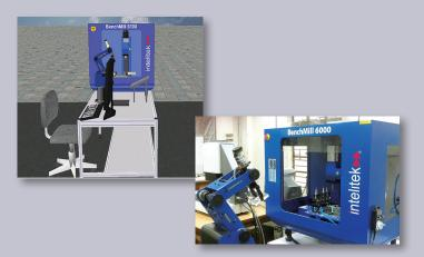
The FMS course teaches students to integrate and operate the industrial workcell. Students develop and edit programs, record precise robotic positions, accurately mill parts, and synchronize mill and robot operation. Students gain "virtual hands on" experience in CNC and robot programming, especially in I/O commands.
