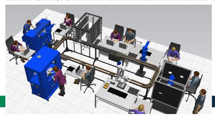
The SmartCIM4.0 is the core of the solution. SmartCIM4.0 is a full-size manufacturing production line with stations designed to manufacture parts from raw material, assemble products and test them for adherence to quality control standards. The solution above is a six station example. This is a flexible model and can be constructed with more or less stations to suit the needs of the school and the program being installed.
